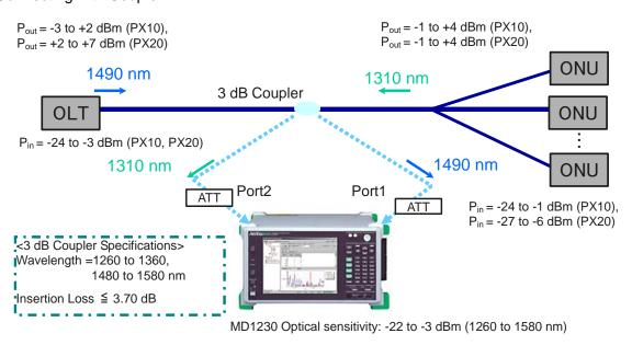
Insert a 2 x 2 coupler between the OLT in the PON system and splitter. Here the coupler is connected directly after the OLT.
