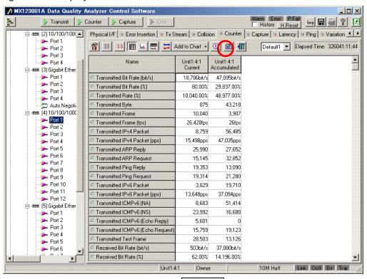
Press the "Display Option" icon at the □Counter screen to open the setting screen.
