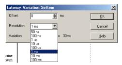
Select "1 ms" at "Resolution:" and press "OK" to close the screen. (This enables measurement of the Latency distribution up to 30 ms with 1 ms resolution.)
