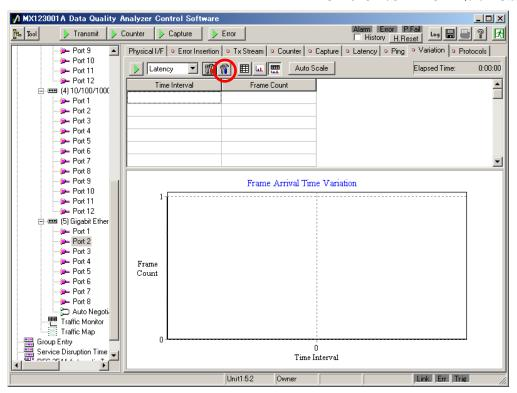
Press the setting icon (blue hammer symbol) to open the setting screen.
