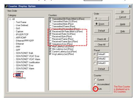
Set which measurement items are to be displayed by placing checkmarks. Here, select "Flow" at "Category:" and place checkmarks at "Received Bit Rate [Mbit/s] (Flow)", "Received Rate [%] (Flow)" and "Sequence Error" at "Counters:". Select "Both" at "Counter". (This permits monitoring of each flow in 1 second intervals using the multiflow counter.)
