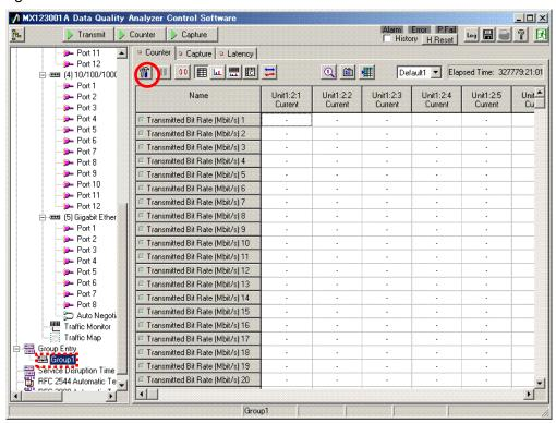
Select Group1 and press the Custom counter display setting button (blue hammer icon) at the Counter screen to open the screen.
