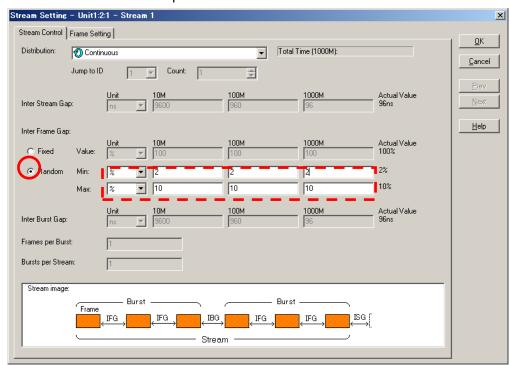
> Select "Random" at "Inter Frame Gap:" and set 1% at "Unit" of "Min:" and 10% at
