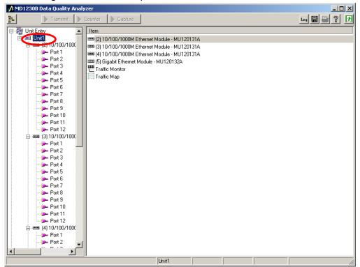
➤ Right-click Unit1 and select "Reservation..." . The ports of usable modules that can be used are listed as shown below; place checkmarks in the required ports and press the "Check all" button.
