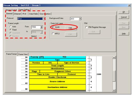
Put a checkmark in VLAN and press "Edit...". The data transmission priority can be increased by increasing "User Priority:". Here set the priority to 7 so as to secure the band maximum priority. (Doing this guarantees the band required by ONU1 and divides the remaining band into 31 equal parts for ONU2 to 32.)
